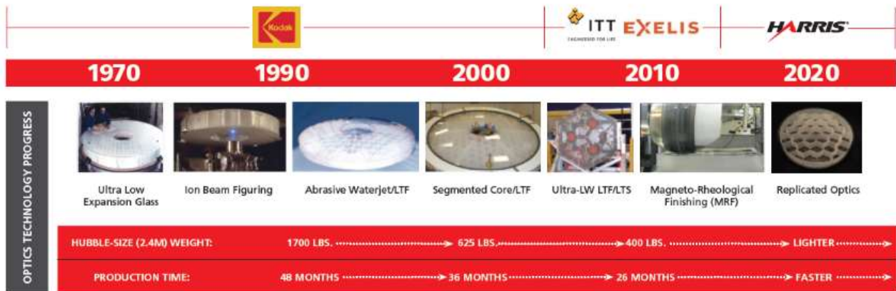
Figure 1: Harris innovation of more than 50 years to advance lightweight mirror technology for both space- and ground-based optical systems through design and manufacturing processes to reduce timelines and cost while meeting demanding requirements.
