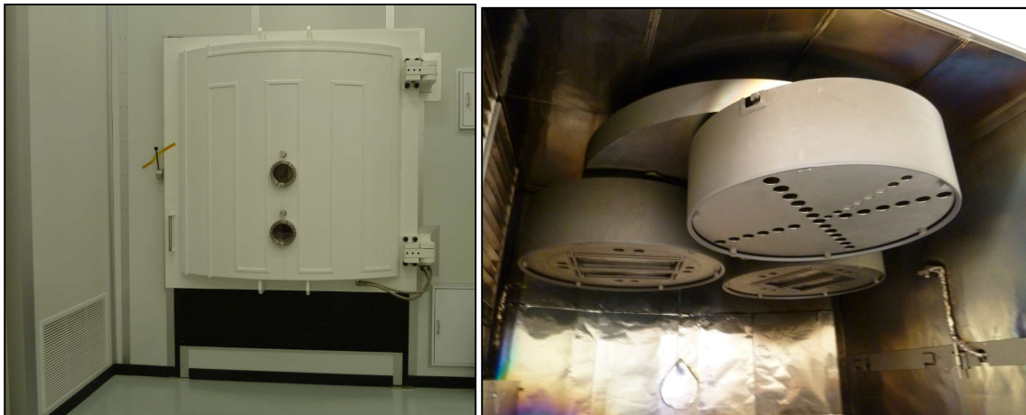
Figure 13 Collins 72" optical coating chamber can be configured for single rotation (1.5m capacity) or with (3) 28" dia planets. Similar chambers are available in our Danbury facility for coating mirrors up to 2.5-meters
